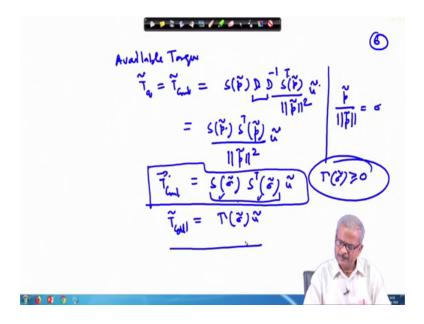
So, the available torque then T q tilde or T coulomb this can be written as we have use the earlier equation. This part we have broken up and this we have written as s p tilde and m we have written as D times q tilde. So, we need to replace here q tilde.
