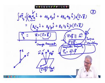
So, this d T q then we can write as let us say that the total distance is from what this is d along the x axis times i cap, ok. And d q which is multiplied there, we will bring this d q here in this place and this is along the x axis, ok. So, d q x times distance along the x axis this two can be added together.
