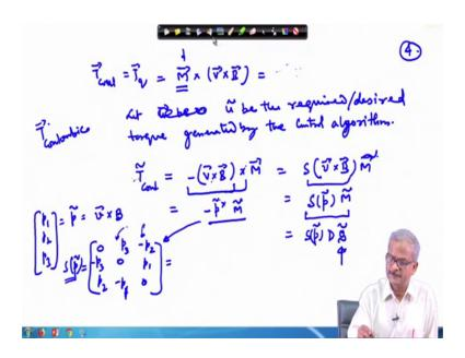
So, we have the torque then we can write as so, T q or this is the columbic or T q we can write it this way, this is T columbic. So, these we can write as already we are written M cross V cross B. Now let u be the or u tilde, you can write in terms of u tilde also, u tilde be the required slash desired torque generated by the control algorithm. So, from there how much M is required we can find it out.
