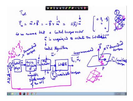
So, the T; the torque due to the magnetic moment; T coil also we can write this as the T coil this is given by m cross B and which we can write as minus B cross m. And as per the skew symmetric matrix notation, we are using. So, we can write this as S B tilde times m tilde; where S B tilde is your skew symmetric matrix as defined earlier. This appears with a B z, here plus sign it will become plus and minus B y here in this place and so on.
