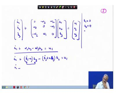
Say h 1 dot h 2 dot and h 3 dot this is for the CMG motion and; obviously, this is a simplified version because we are neglected the internal and the external gimbal mass, if we do not neglect it then the for the double gimbal variable speed control movement gyros whatever the procedure we have followed that procedure needs to be followed and thereafter the control has to be designed, so u 1, u 2 and u 3.
