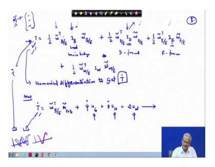
And if you are simulating the equation of motion, so we you need to verify that your equation is working alright. So, how to verify this? So, for that you need to write the kinetic energy. So, kinetic energy will be written as, so this is of the main body ok. Then you have to take into account the outer gimbal and then you have to take into account the inner gimbal which we have written by F.
