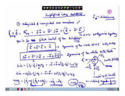
So, under the assumption: that outer gimbal and inner gimbal are mass less. So, therefore, their motor will also not be considered the outer gimbal and inner gimbal are mass less. So, under this assumption we have simplified the equation of motion as M external this equal to I times or the J times, where J is the angular momentum of the moment of inertia of the whole body. This h is with respect to the body axis, this we have derived earlier body axis system; body axis body axis system.
