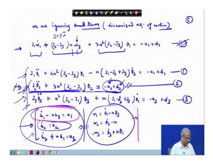
So, the first equation we need to reduce and put it in a proper format. So, what we are doing that? We are ignoring small terms and after ignoring it we whatever the equation we get that becomes our the linearized equation of motion. So, from here we get the linearized equation of motion. This is the gravity gradient term that we have brought it on the left hand side and this is the term omega tilde which is appearing from omega tilde cross J times omega tilde.
