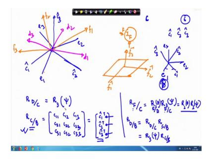
So, what we see that, my body frame is located here. This is e 1, e 2 and e 3. With respect to then we have the, somewhere the even frame here in this directions c 3 cap and c 1 cap, c 2 cap these are located ok. This center they are matching it is a little poor figure with respect to this c 1, c 2, c 3 your d frame is oriented, ok. So, d frame is oriented somewhere say for that we can draw it by other color. So, this is your say the d 1, this is
