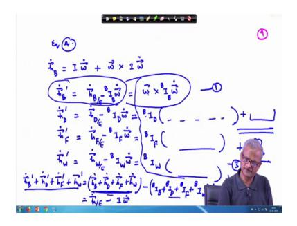
So, the equation A, now we can rewrite this as that was for h body, h dot body this equal to I times omega dot plus omega cross. We define a new quantity h B dot prime and write this as h B dot minus I omega dot and this equal to then right hand side becomes I times omega dot. Let us say this is equation 1.
