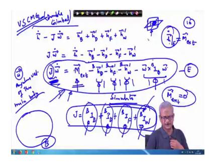
So, we go on the next space. So, what we have got here, I times omega dot and then h dot minus I times omega dot, this quantity is equal to h B prime h D prime all these things. So, this is h B prime plus h D prime plus h and then F prime, little bit of rearrangement of this is required. This is the angular velocity of the satellite as we have said earlier omega is the angular velocity of the main body which is nothing but your satellite bus or the outer portion which we have indicated by B.
