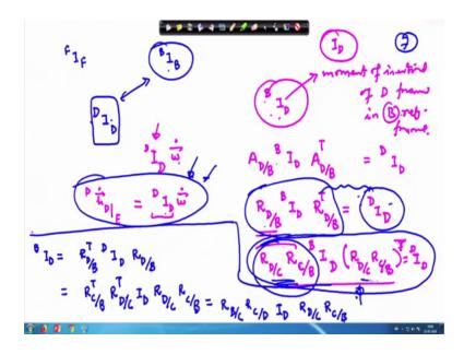
Now, the equations already we have derived, however as we have seen that the moment of inertia we are of the F frame we have defined in the F frame itself ok, while for the moment of inertia of the body we have written along the body axis. So, all this equation A, B, C and D this is in a different frame; this is in obviously this we have done this is in a different frame ok.
