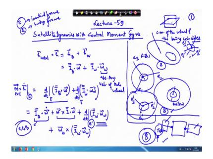
So, if you remember, we wrote h total or this h the total angular momentum of the satellite, we broke into two portion. One is this satellite which we have written by this b and inside, there is a hollow and in this hollow the control moment gyro which is located there and we are showing like this.
