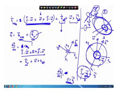
So, we have here h dot total this becomes equal to j double bar dot omega, plus omega cross j double bar dot omega and this constitutes your satellite part along with the CMG. CMG is also there and this is the main body is also there and this is the wheel. So, that is also present. So, those two things are combined together and the other part we are writing as h s dot plus omega this part we have combined here. So, other part omega times hs ok. So, this is omega times hs.
