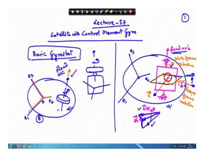
So, in a basic gyrostat what we have that there is a satellite body main body which we have written as B, and inside this there is a wheel which is rotating on it is axis, but this axis remains fixed which we are showing, as a or either we are considered at the same thing can be something like this. I have a satellite and outside this there is a wheel. So, this wheel is rotating about this axis ok. So, it is rotating this wheel is rotating.
