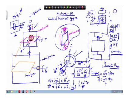
So, usually the control moment gyros pa earlier also I have talked about this. So, control moment gyros it looks like we have a say frame here, and this we call as the gimbal axis for this frame, then we have another frame -and there is a wheel what we call as the rotor and this is the rotor -and from the centre of this rotor, this conduction goes back here and comes here in this place.
