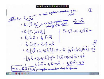
So, h a we can write as also e a cap times angular momentum of the wheel; remember this is the absolute angular momentum, absolute angular momentum of the wheel. Because we are discussing about this figure this is the free body diagram, this is the free body diagram. This is also a free body diagram.
