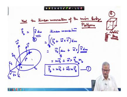
Linear momentum of the main body, this main body also this is called the platform.. Sometimes the also the casing of the satellite say this is a satellite, so, this is the satellite casing. So, this is basically a honeycomb structure means the casings are made of panel which inside just like the honey bee is having it is high. So, the same way this structure is there. So, you will see if this is hollow, and on the 2 sides of thin plates are pasted to make it light and also give it a strength.
