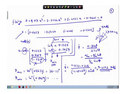
So, once we expand we get the following equation 2.6487 x cube this equal to 0 and in the MATLAB you can defined a vector a tilde like this just give the notation in the MATLAB. a equal to 2.6487 live a gap give a space then 7.5066 then again give a space 5.6021 copy all these coefficients here give a space and then 9.421, and then give command roots a. So, it will list you the roots of this polynomial ok. So, this is your polynomial f x; f x equal to 0 you are solving.
