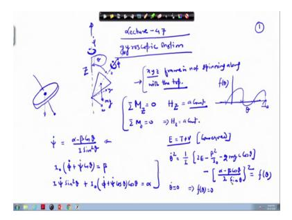
The difference lying that in the case of the gyroscope because the centre of mass it may happen that like you are considering a wheel, ok. So, if it is a pivoted about this point then there will be a torque acting, but if it is pivoted about this point itself about the it is a centre of this disc. So, in that case there would not be any torque, so, that will become a torque free case.
