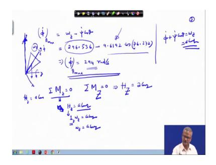
Then we also need to calculate phi dot phi dot corresponding to theta max. So, this quantity will be omega z minus psi dot cos theta and omega z already we have computed. This corresponds to theta max. One thing you should note here that along the z-axis of the cone your omega z is here, ok. This is the z body axis and x body axis is here, y body axis is here. So, omega z we have written phi dot is also along the same line.
