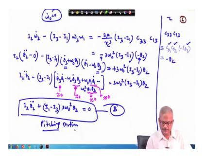
Let us go in the next page and then workout. So, we have I 2 time omega 2 dot minus I 3 minus I 1 times this is the earlier I have told how to write this equation. You do not have to remember in this one this is just a in a circular order. So, we can write it that way only omega 3 omega 1 minus 3 mu by r c cube times I 3 minus I 1 and c 3 c 1 and then write 3 3.
