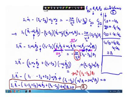
Now, we can write the Euler's dynamical equation. So, I 1 times omega 1 dot minus I 2 I t 3 I 3 times omega 2 times omega 3, this equal to minus on the right hand side we have the torque equation, because the torque term because of the gravity gradient term, which is minus 3 mu by r c whole cube ok, this we have done earlier times I 2 minus I 3.
