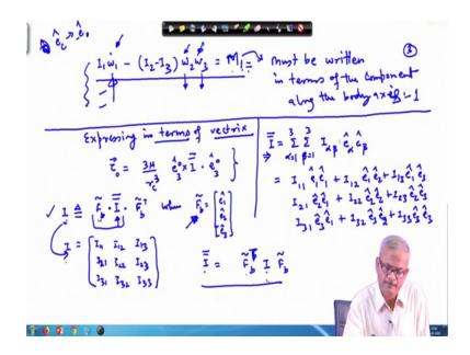
So, if you remember that the Euler's equation, we have written I 1 times omega 1 dot minus minus I 3 times omega 2 time omega 3 equal to the torque on the right hand side which is in M 1. Similarly, the other three two equations ok. So, here omega 1, omega 2 which are appearing so, these are the components of the angular velocity vector along the body axis direction ok.
