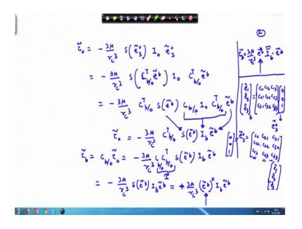
So, we have tau tilde o, this quantity equal to minus 3 mu by r c whole cube, and then s times e tilde o 3 times I o. Then we will start writing this as c transformation from orbital frame to body frame I 0 c transpose b slash o ok. And this can be written as c transpose b slash o, and this quantity is nothing but your I b. This converted into the body frame as I have discussed earlier ok, rest we copy it from this place ok. Here we have not written it correctly.
