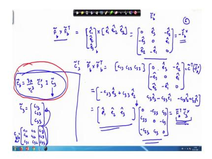
So, F b tilde cross F b tilde transpose, now this is the e 1 cap e 2 cap e 3 cap. This is all along the body or direction which I may not write it, because it is unnecessary to carry
