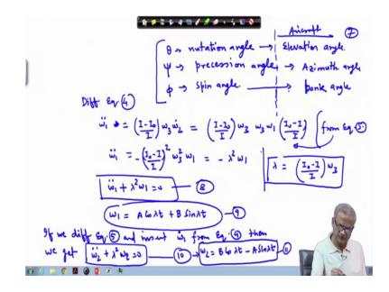
As I have told you earlier this theta, this is called a nutation angle, psi dot its called the precession angle and this psi is called the precession angle not dot and phi this is called the spin angle. In the case of the aircraft the same thing is called as the elevation angle, this is for aircraft. This is precession angle instead of this precession angle, we write this as the azimuth. And, this spin instead of this phi elevation azimuth and then elevation
