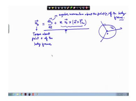
So, the final conclusion what we get is dh b by dt plus M times V 0 cross omega cross rho cm and this quantity is nothing, but equal to M b where M b is the torque about the body frame. So, this is the torque about point O of the body frame and h b, this is the angular momentum about the point O of the body frame ok.
