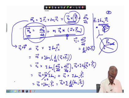
So, what we have got? This is M b equal to rho i cross delta mi times V i summation over this. This is nothing, but equal to V 0 cross P. This is the linear momentum of the body and plus dh b by dt. This particular term can be further expanded. So, we have V 0 cross P. Now the quantity P that we have written, this is delta m i times V i delta mi times V i and summation over the whole body, this is what we have written.
