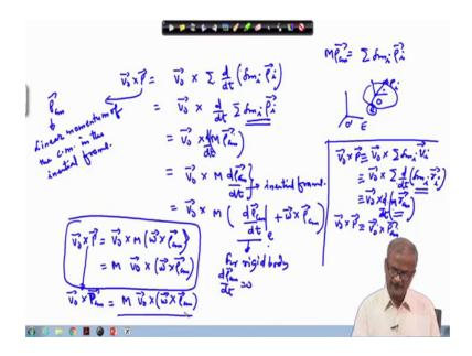
So, we have V 0 cross P this is equal to V 0 cross summation d by dt summation d by dt and delta m i times rho i. Exchange this operator and you know that this quantity is nothing, but the location of the centre of mass. It is relate to the centre of mass. So, this is M times rho c m and then we have d by dt. So this gets reduce to V 0 cross M times d rho cm by dt.
