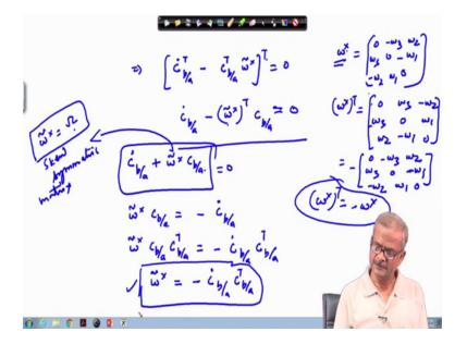
So, this implies if we take the transpose of these whole things. So, c dot transpose b slash a minus c transpose b slash a omega tilde cross take transpose of this, this must be equal to 0. And if we take the transpose, so this gets reduced c dot b slash a minus omega tilde cross transpose times c b slash a; this equal to 0. Now this quantity you know this is the
