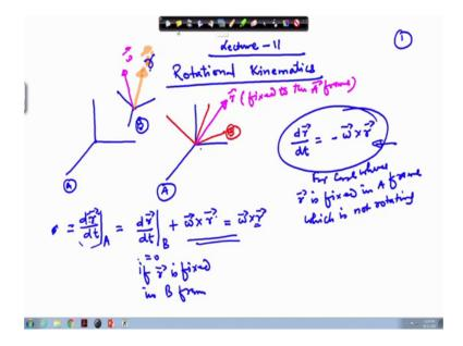
Say I have a frame here which I write as A frame and another frame which is the B frame here. This B frame may be located here at this point the origin of both of them we can locate here and we can show it like, this is the A frame and the B frame it looks like this; this is the B frame. So, A frame has rotated to B position and let us say that we have a vector r which is fix to the through the A frame.
