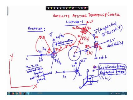
So, let us start here. So, let us consider that we have the earth here; it can be any planet or natural satellite of that planet. And there is a satellite here in the orbit; this is orbit. And satellite velocity vector can be represented as v which is tangential to the orbit ok.
