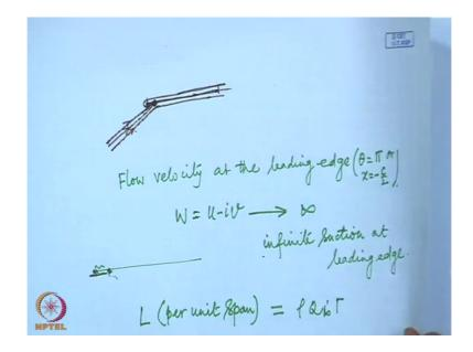
I mean, the flow pattern. First of all, think that this is what is our flat plate; the flow is coming at an angle alpha; the forward stagnation point is somewhere here on the lower surface. Let us say it is somewhere there. It is on the lower surface; it is not at the front point; it will it will be at the front edge when alpha is zero; for any non zero alpha, it will be on the lower surface assuming positive alpha.
