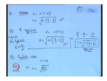
So, if the equation that we have derived this is for an ellipse for an ellipse we have a is equal to 1 is equal to a times 1 minus a square; therefore, for an ellipse the v will be given by mu times 2 by r minus 1 by a if the we have hyperbola. So far that the one will be given by a times c square minus 1, so the result will get reverse and here the change of sign will take place.
