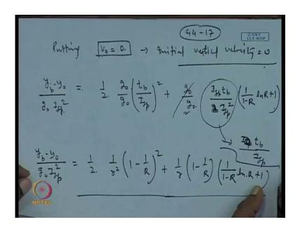
By putting v 0 equal to 0 that is, initial vertical velocity is 0. So, this becomes y b minus y 0 is equal to 1 by 2, we divide both the sides by g 0 I s p square. So, this will give us g 0 t b by I s p square plus g 0 by g 0 and I s p time t b, we have, we can insert from here. So, this is I s p times t b divided by g 0 g 0, we have already taken here into account this I s p square times 1 by 1 minus R 1 n R plus 1.
