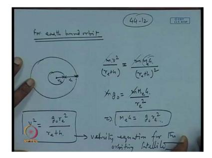
Now, for earth bound orbit let us calculate the required velocity, we can write a very simple equation this is the earth. So, here this is your radius of earth r e and this, we will write from here to here this is the altitude. So, m v square by r e plus h the necessary, centripetal acceleration is provided by the gravitational force. This we cancel out and here also this term will cancel.
