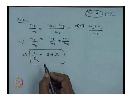
Also, we can write m b by m 0 is equal to m s plus m l divided by m 0 and this becomes m s by m 0 plus m l by m 0. So, this will be left hand side is 1 by R and m s by m 0. This is the dead weight fraction s, we have written as an m l by m 0 as l. So, this is another relationship we are getting.
