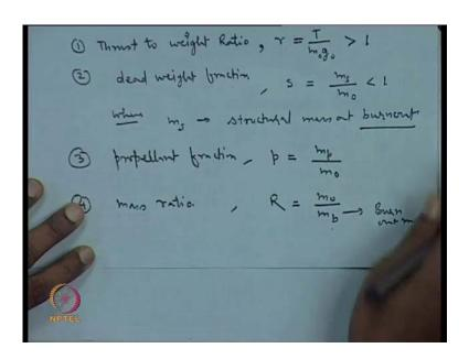
So, we define some design parameters such as, Thrust to weight ratio and this quantity is greater than 1, dead weight fraction s and we define as m s by m 0 and this quantity is less than 1. Where, m s is the structural mass a structural mass at burnout.
