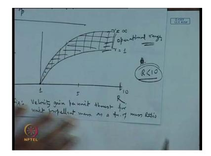
So, your velocity remains finite. So, this is your operational range basically, operational range we cannot go beyond this range and we have to work with in this limit where, as I already told that R is generally less than 10. So, this figure, we will term as the velocity gain means v b minus v 0 is your velocity gain per unit thrust for unit propellant mass as a function of mass ratio.
