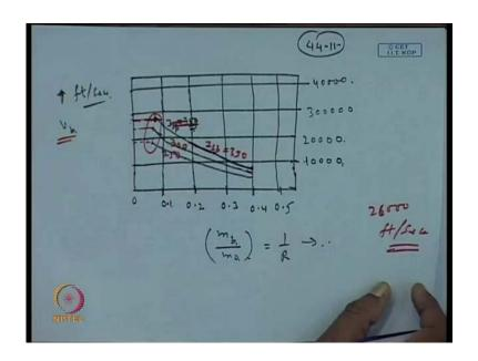
So, now one more figure, we will draw if, we plot the burnout velocity on this axis in feet per second and m b by m 0, which is nothing, but 1 by R. On the axis. So, you will get, some this kind of plot that on this axis let us say, this quantity is 10000; this is 20000; this is 30000 and here, this is 40000.
