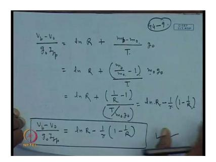
Now, divide the numerator, denominator by m 0 in this term. So, this is m 0 by m b divided by m 0 minus 1 m divided by t divided by m 0 let us, written on a separate page g 0. We can put here, and t in this place. So, this is m b not m 0 now, dividing this by m 0. So, 1 n R plus m b divided by m 0 minus 1, this becomes m 0 times g 0 divided by t. So, 1 n R plus m b by m 0, we know that this quantity is equal to 1 by R, this is minus 1 and t by m 0 g 0, we have written as the thrust ratio.
