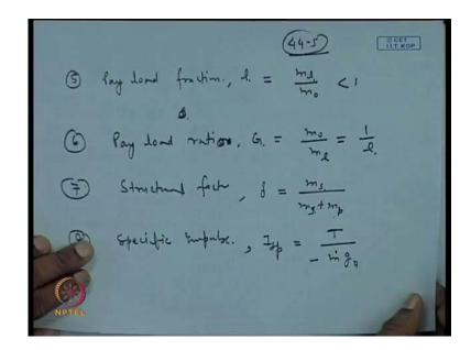
So, these are the design parameters of a rocket. Now, m 0 can be written as m pay load plus, m propellant plus, m structure mass. Now, at the burnout all the propellants will be burnt. So, we can write, this as m p plus m l plus m s and this is nothing, but mass of the rocket at the burnout m b and this is the mass of the propellant. So, m b is nothing, but m p plus m s. So, what we have written here m b is m s plus m propellant.
