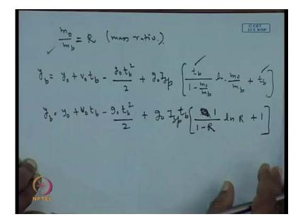
This is what we get in the now, to do further simplification, we just put m 0 by m b equal to r, which is the mass ratio. So, this gives us y b equal to y 0 plus v 0 t b minus g 0 t b square by 2 plus g 0 I s p. I am dividing this term, m b in the numerator and the denominator dividing by m b. We get here, as the t b and in the denominator 1 minus m 0 by m b and similarly, m 0 by m b plus t b.
