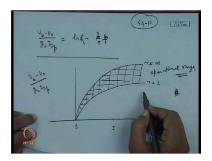
So, this equation for v b minus v 0 by g 0 I s p, this can be also written as 1 n times 1 n R minus 1 by r 1 by r minus times p 1 by r times p. Now, we can if we draw a plot for this by plotting r on x axis v b minus v 0 and divided by g 0 I s p on the y axis. So, this we take as y and this as the x and this as the parameter. So, in this you look in this equation basically, we are trying to plot this equation. So, here minus 1 by r is appearing multiplied by 1 by r.
