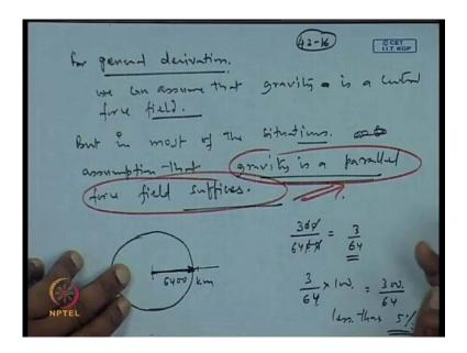
So, for general derivation, we can assume that gravity is a central force field, but in most of the situations assumptions most of the situations or assumption in most of the situation or assumption that assumption that gravity is a parallel force filed suffices. And, reason for this is say your earth, is it is a radius is around 6400 kilometers. While you will be launching, and inserting the satellite at an altitude of 252 to 300 kilometers, so you add an altitude of 250 to 300 kilometers.
