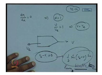
And, for maximum efficiency then, dou eta by dou alpha. You set it to zero differentiate this quantity, and this will imply you alpha equal to one. So, alpha where set as v by v e. So, this is equal to one this implies v equal to v e, which is the same thing just by observation, what we have written here. So, in this situation what is happening that rocket is moving with velocity v in this direction, and exhaust is coming out of this.
