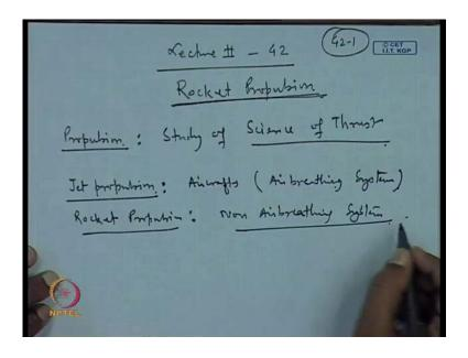
So, in the propulsion we define this as the study of science of thrust. So, we can have various types of propulsion like we can say the jet propulsion, which is nowadays used on aircrafts, and this is basically air breathing air breathing system. While on the other hand the rocket propulsion, this is non air breathing system. Still now, but scientists are trying for air breathing rocket propulsion also.
