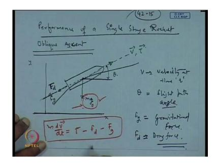
So, proceeding with this assumption that the gravity is remaining constant, so here we will put instead of g. We will put here g 0 to indicate, this is the gravitational acceleration at the surface of the earth. Now, we can see that as the as the rocket goes up. So, this the value of the g, becomes small, but here the distance change is not much. So, that the change will be no appreciable, and we will not be making any mistake or doing a very large mistake by making this assumption.
