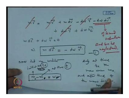
Now, we can see from here this can be cancelled, and d w v is here with minus sign. So, this can be cancelled out this quantity, this is of second order. So, d w is also infinite simply a small, and d v is also infinite simply small. So, both of them together it constitutes second order term, and can be neglected. So, what we get from this place m d v plus d w times v this is equal to zero, and this implies m d v equal to minus d w v.
