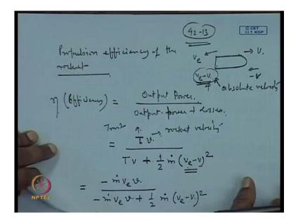
So, another equation in this connection, we can write the propulsion efficiency of the rocket propulsion efficiency of the rocket. So, this we write as, it eta this is the efficiency and this is the ratio of the output power by the total power. So, this is output power total input power, so output power plus losses.
