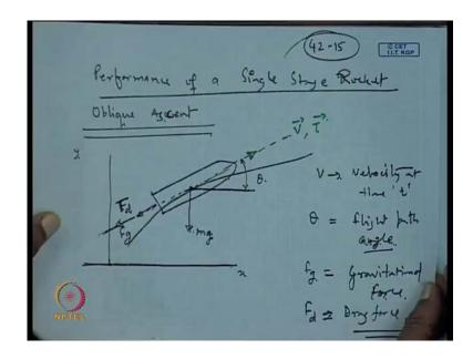
Now, once we have done this. So, we can now develop the equation for rocket performance in single stage. So, single stage rocket performance of a single stage rocket, and we write a general equation that is for oblique ascent say this is our inertial x.
