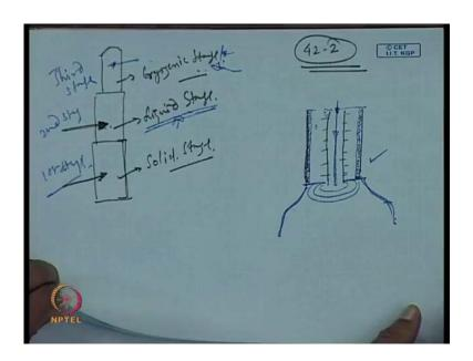
So, a rocket can have a number of stages. So, in general we will see that, three stages may be applied. So, this stage may be the solid stage or the solid rocket and this is the liquid stage and this is this the cryogenic stage. In the liquid stage some different materials can be used, some hydro carbon or other materials can be available. While in this case the solid propellant means; in the rocket the solid propellants are first mixed with some blue, and then it is packed inside the rocket.
