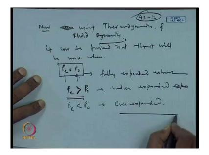
Now, using thermodynamics and fluid dynamics, it can be proved that thrust will be maximum. When p e equal to p zero, that is exhaust pressure equal to the ambient pressure, and this is called fully expanded exhaust. If, p e is greater than p zero then, this becomes your under expanded. So, still it is not fully developed the flow is not fully developed.
