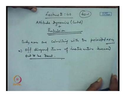
So, what last time we worked out that a rigid body is given and the body axis are coinciding with the principle axis. So, our assumption was body axis are coinciding with the principal axis. So therefore, the off diagonal terms, off diagonal terms of inertia matrix turned out to be zero. And then, we worked out the equation of motion using the Euler's dynamical equation by setting the torque in that equation to zero.
