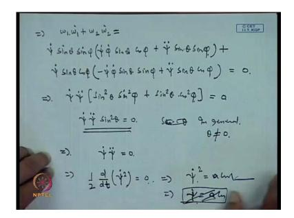
So omega 1 times omega 1 dot. So, we have omega 1 psi dot times sine theta and then we put the omega 1 dot value, just now we have expression we have derived. Psi psi dot times phi dot sine theta Cos phi plus psi double dot sine theta and sine phi and plus omega 2.We have written as psi dot sine theta times Cos phi and this to be multiplied by
