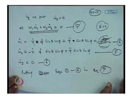
So, if we put omega 3 dot equal to 0, so this implies omega 1 times omega 1 dot plus omega 2 times omega 2 dot this is equal to 0.And just now we worked out the relationship for omega 1 omega 2 and omega 3 so these are available to us. And, what we need further, this is omega 1 dot omega 2 dot. So, omega 1 dot we can use the
