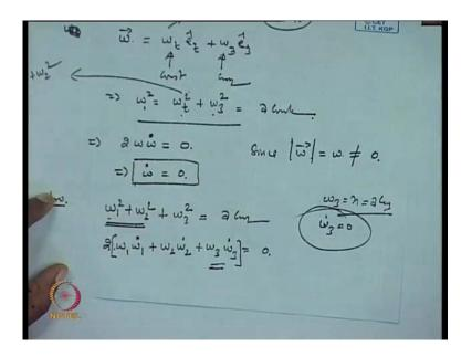
So we have, now let us get back into the omega vector which we wrote as omega t times e t cap plus omega 3 or n times e 3 cap, where omega t is a constant omega 3 is constant.
