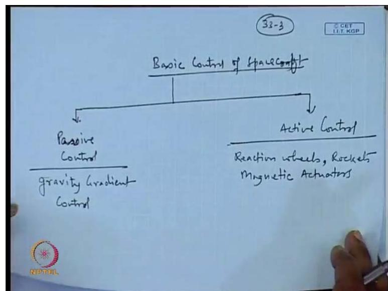
So, let us consider that some basic aspects of the satellite attitude control. So, we will have the basic control of spacecraft this we can broadly write has the passive control. So, in the passive control we have the gravity gradient control in the active control we can cut our eyes like the reaction wheels the rockets. So, rockets are of various types again then the magnetic actuators. And also we can list in this the dual spin dual spin system. So, we are going to discuss all of them briefly.
