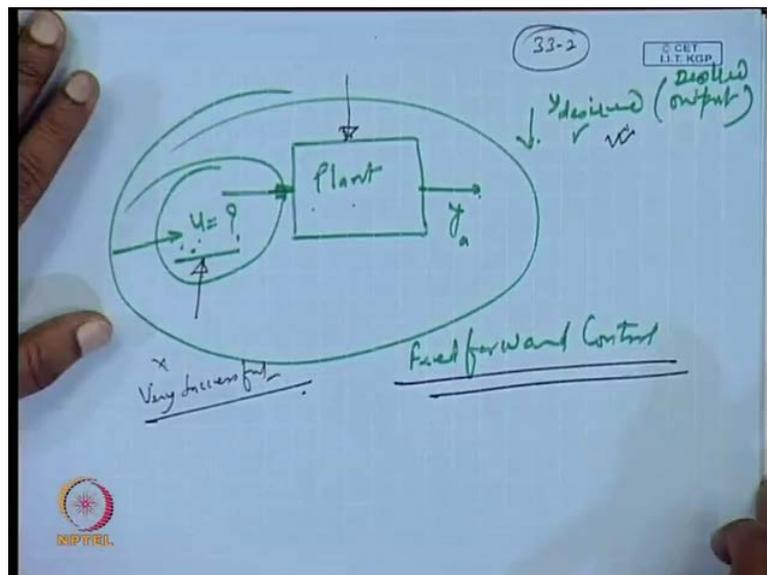
So, in the control system the objective remains given the plant and say desired output. So,  $y$  desired this is the output desired output and  $y$  say  $a$  is the actual output. So, you design the control inputs. So, basic objective is to design this inputs in such a way that you achieve the desired output here so; obviously, if your plant is a dynamical system. So, in that case you can design your inputs to the system or to the plant or priory and this is called the feed forward control.
