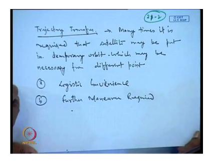
In Trajectory transfer many times it is required that satellite may be put in a temporary orbit. This may be quite necessary from the point of view that while you are launching the satellite, so at the time of the ejection from the rocket while you are injecting it in the orbit at that time it goes under severe conditions. So, after the injection then you may be
