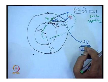
In the non tangential burn, again this is the center of the force satellite is moving in this orbit and I need to put it in a higher orbit. So, it is possible that I can give an impulse here in this place. Here, suppose this is your velocity vector v circular in the initial orbit and I can send it along any of the trajectory. I can send it like this or either I can send it in this orbit, I can send it here this way various possibilities are there.
