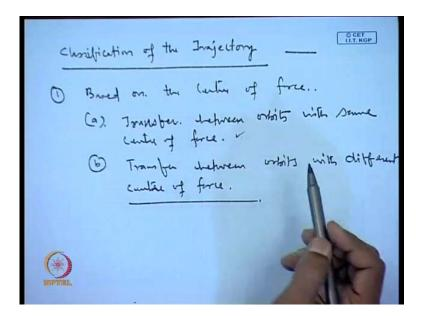
Now, the classification of the trajectory - the trajectory transfer, we do it can be done based on various factors. The first we decide on the basis of centre of force. So, here we can have transfer between orbits with same center of force transfer between orbits with different center of force.
