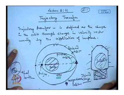
So, to start with trajectory transfer is defined as the change in the orbit through change in velocity vector usually by the application of impulse. So, often one or more impulses will be required to complete the trajectory transfer. Let us consider a very small case.
