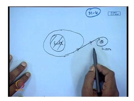
This is your earth and here is the moon. So, you have placed the satellite in an elliptical orbit and you want to capture it around the moon. So, you can give impulse in this orbit and it can be brought like this. Thereafter it can be captured.
