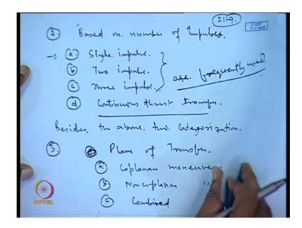
The second categorization can be done based on the number of impulses. So, we can have single impulse transfer. This is your first the minimum possible and two impulse and three impulse continuous thrust transfer. Of course, these three are frequently used.
