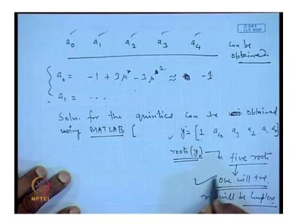
So, once we have got this mu star then the coefficients a 0, a 1, a 2, a 3, a 4 can be obtained. Because the equations for this coefficients a 0, a 1, a 2, a 3, a 4 we have already written. You just need to insert the value of mu star and compute it. This can be done in MAT LAB very easily. But the MAT LAB, it does not give you very accurate calculation unlike if you program in Fortran or C and use double precision there.
