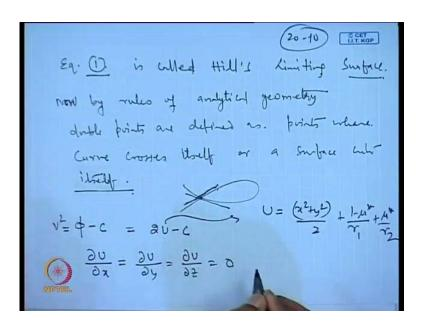
So, this equation 1 is called Hills Limiting Surface. Now by rules of analytical geometry, double points are defined as points, where curve crosses itself or a surface cuts itself. So, double point will exist here in this place. So, you will have two tangents here, one like this and another like this. So, double points.
