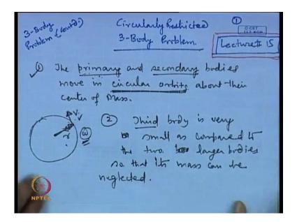
So here, the primary this is assumed to be quite large as compared to the secondary body and the third body, it will be assumed to be quite small as compared to this primary and the secondary body and so that it is mass can be neglected. So, mass can be neglected and the third assumption which is again which gives further restriction can be made or sometimes it is a made is that.
