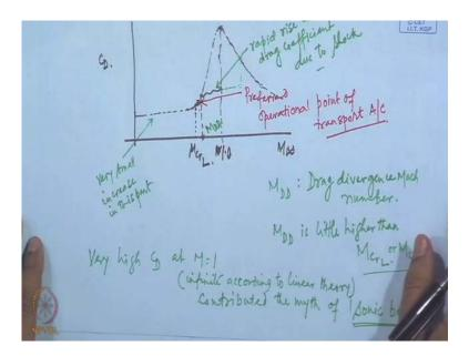
So in this case, rapid rise in drag coefficient in to shock and we also have defined, what is the divergence drag? Divergence Mach number, where the shock wave becomes started contributing largely to the drag coefficient, that becomes the drag divergence Mach number. Now, it a very important to particularly, estimate this lower critical Mach number, because it is that more or less fixes the preferred operational point or cruising speed of a particular aircraft.
