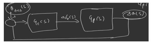
So, we can apply this concept to come up with the transfer function and if you are having transfer function we can design the control algorithm. So, here we are having  $\Delta \theta(s)$ , this is the controller which is giving the control input to track  $\theta_{des}$ .
