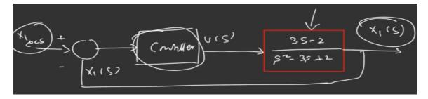
This is how we can design the controller here and this control will track help to track  $X_1(s)$  to  $X_{des}$ . So, this part already have done in the first half of this course how we can design the control system if you are having the plant in transfer function form. So, let's stop it here we will continue from the next lecture we will come up with different system and how we can come up with the transfer function so that we can apply the linear control techniques. Thank you.
