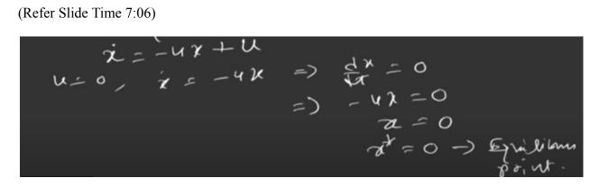
So here to find equilibrium point  $\frac{dx}{dt} = 0$ , we can make it zero. And from this -4x = 0, so x = 0. So in this case,  $x^*$  is zero, we can assume an equilibrium point. So in the LTI system, most of the LTI system or equilibrium point is assumed to be at origin  $x^* = 0$ . So now we'll shift our attention, how we can look at this concept of equilibrium point for an aircraft.
