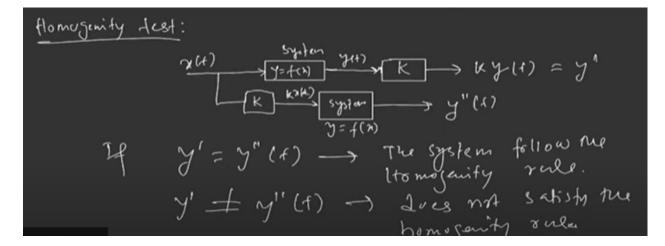
Let's take an example, which can validate the above theory. So, y = f(x), and the f(x) function is  $\frac{x^2}{16}$ . We will say the system is linear or not. So, we will go two tests, one is the homogeneity test, another is the additivity test. First, let us go with the additivity test.
