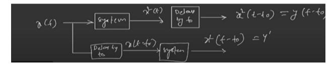
The system is time invariant. It is good that the system follows the time invariant properties but the system does not follow the linearity property. So, the system is not linear, but time invariant. So, this is how we can check if the system is LTI or not, system is time invariant or not, system is linear or not. So, this is how we will be doing. So, now in the next lecture we will be talking about why we have to consider the LTI system for designing control.
