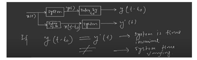
If it is not satisfied, then we can say the system is time varying. So, this is how we can check the system is time varying or not. Here, basically, most of the systems where the coefficients are assumed to be constant, basically, those kinds of systems are time invariant systems. Now, let us take an example that I think will probably be clear. Example, y(t) = t x(t).
