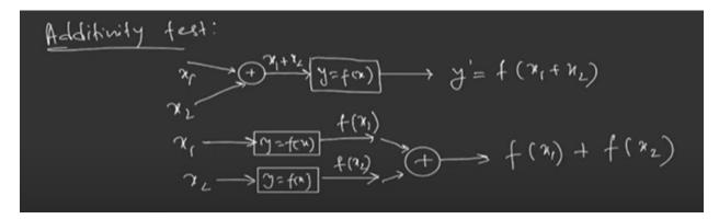
Now if y, let me write this y''. If y' = y'', we can say the system follow the additivity rule. And we need to go to the second test which is the homogeneity test. In homogeneity, let's consider the same system y = f(x), this is my system. And let's apply input which is x(t).
