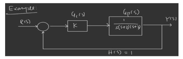
So fiR(s)t example, and we are having summing point here, giving the reference input R(s), and we are assuming there is one controller which is gain k, this is  $G_c(s)$ , and this output of this controller goes to the plant, and this is the output of this plant Y(s), and the output is feedback to the summing point through the unity feedback, and here the OLTF we can come up, the OLTF,
