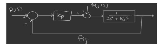
We are having summing point here and we have reference input R(s) and we'll look the modified pd control attitude system so it is  $k_p$  is here and we are having disturbance on the system  $M_d(s)$  which is we can say constant. We'll assume the constant disturbance acting on the system and we have the modified plant transfer function
