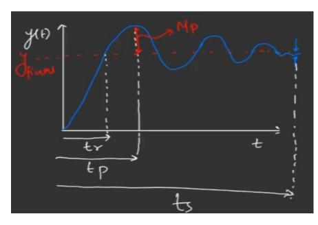
So from the step response, let me define this the figure 1, from the step response in figure 1, we see that at  $t = t_r$ , the output is y(t) equal to 1. Hence, if you remember the equation we had,
