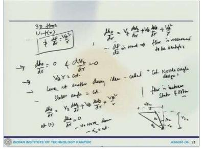
Now, once we look at the 3D flows since the blade velocity U is function of r the velocity triangle changes from root to tip of the rotor obvious the reason, the flow properties also vary with r and the radial equilibrium condition has to be fulfilled which is
