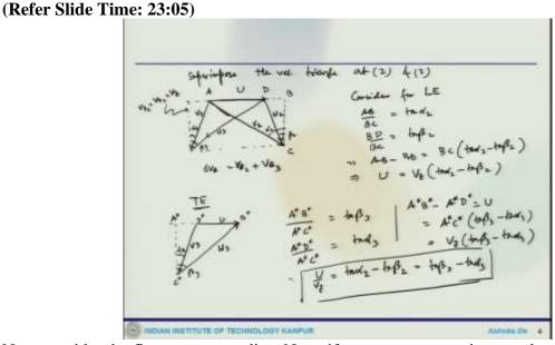
Now consider the flow at mean radius. Now, if we suppose superimpose the velocity triangle, let us say superimpose the velocity triangle at 2 and 3. So, which will look like we have this component now like this that goes here. So this is U. So, this is U this is  $W_2$ , this is  $V_2$ . Now, this is point A, this is let us say point B, this is point B this is C and this is  $\alpha_2$  and this is  $W_3$  and this is  $V_3$ .
