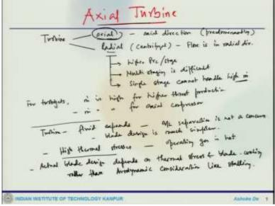
So what we will start doing that we will look at the axial flow turbine. So this is what we are going to talk about, but at the beginning, let me again reiterate that fact. That turbine also could be 2 types. That means it could be axial or it could be radial. So, which; is sort of what we talked about centrifugal compressor. So, this could be radial and this could be also axial. So we will start with the discussion on the axial turbine.
