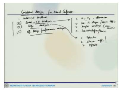
Now, one can think about some conceptual design, how to get it for axial compressor so, typically the compressors are designed by indirect method. So, the first one defines the flow path that means casing and half radius and decides the thermodynamics aerodynamics forces. And then the flow path and iterative analysis is conducted the continuity momentum energy equation for such conceptual designs.
