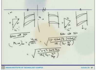
So, we can see how I mean already we have looked at that, but again just to reiterate the fact by showing some so the velocity triangle would be like this. So, this is  $V_1$ , U, this is  $W_1$  and this is  $V_z$ , this is a. Now, that  $V_0$  which goes in, so, these are the blades here. So, when it comes out that comes out this is U, this is  $W_1$ , so that is  $V_{z1}$  and this is U,  $V_1$  then again, so this goes back so that is how the U also. So, this is 2 different scenarios.
