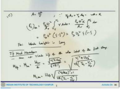
So, we are looking at now the tip Mach number. So, this I said that because this is another important parameter, because the maximum Mach number in the axial flow compressor occurs at the blade tip of the rotor inlet on the first stage. So, this is essentially maximum at blade tip of the rotor inlet of the first stage. So, this is due to the maximum value of the relative speed W 1 and the maximum static temperature of the sonic inlet.
