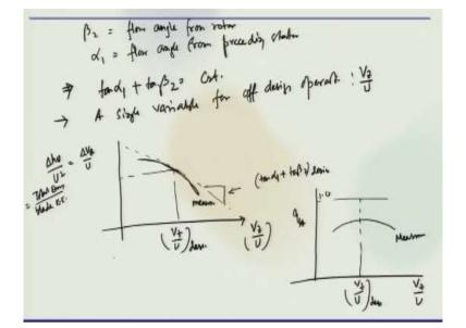
So which means  $\beta_2$  would be the flow angle from rotor  $\alpha_1$  is the flow angle from preceding stator. So in total  $(\tan \alpha_1 + \tan \beta_2)$  is constant. So which assuming this while the entire result of departure from design condition are concentrated in a single variable  $\frac{V_z}{U}$ . So what we get a single variable for off design operation that is  $\frac{V_z}{U}$ . Now we can plot this parameters like this is how we can plot that  $\frac{\Delta h_0}{U^2}$ .
