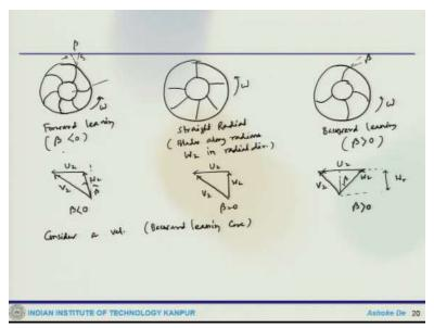
One possible is that you can have like this kind of blade arrangement like this, so this goes like this, so this is the angle called  $\beta$  and you can have; then this called forward-leaning where  $\beta < 0$ . So the other case one can have is that straight radial kind of blades. So this is the rotation, so this is straight radial or third option could be the backward-leading that means the blade could be arranged in this direction still the rotation in this direction.
