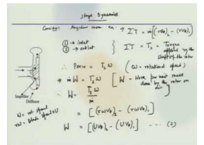
Now, you take the simpler portion and then look at the stage dynamics, so this is centrifugal compressor stage dynamics, now we consider the angular momentum equation which is
