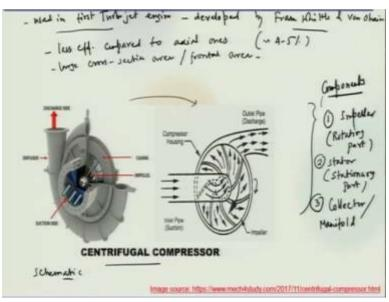
So, this is one of the images of a centrifugal compressor, one can see I mean, it will give you an idea how it looks like, so this is what the inlet side, when it comes in, so this is the another schematic of here, so from here to here you can see this fluid comes in here, goes through this impeller, so these are this what you see here, these are the impeller blades and flows goes through that and finally goes out radially, this is the discharge side.
