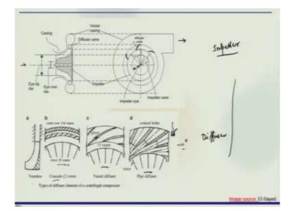
Now, if you look at this portion of the image, this is the portion which you call the I mean, this cut section if you take it, this is how it looks like and this is how the other side, so you can see this is the impeller, this is the shaft, then you have diffuser vane and the side view of that and this is the volute casing, so these are impeller vanes which are here, then tip diameter, root diameter all these different things.
