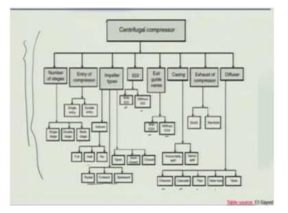
And also now, this if you look at the classification of the different kind of centrifugal compressor, this actually takes into account of lot of the things, I mean it starts with the number of stages, I mean, this one can think about the different kind of components or different type of centrifugal compressor which possibly can be there but then what are the other complications that can have.
