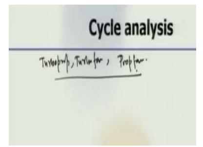
Now, one can compare this like between turboprop, turbofan and propeller fan. So if you compare that propeller fan engines have the best known propulsion efficiency. Single rotation propeller engines have propulsion efficiency around 80%, while contra-rotating can go up to 90%. So main feature of propeller fan engine versus both turboprop and turbofan engines are quite significant.
