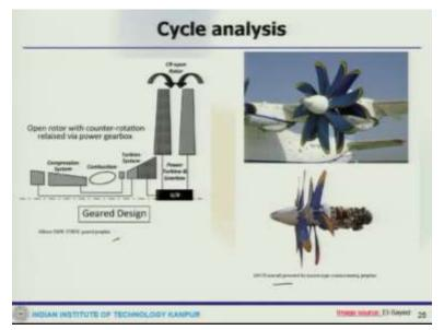
Like this is another one which is Pratt and Whitney 578DX which is 1980. This is also having a reduction gearbox between LP turbine and the propeller blades. So some progress been made. So this is our D27 propeller fan. So this was developed by USSR. So this is even conventional in layout with propeller fan blades in front. So it is used for propelling AN70 aircraft. so this was used for AN70 aircraft.
