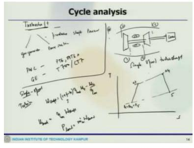
Because what we have finished like the comparison with the turboprop with the turbofan and now we are going to look at the turboshaft. So this is also going to be a small section. This also kind of engine is a form of gas turbine, which is optimized to produce shaft power other than jet thrust. So this produces shaft power not the jet thrust. Generally, a turboshaft engine is made up of two major components; one is the gas generator, another component is the power section.
