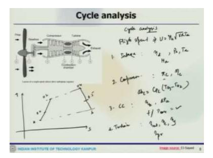
Now this is a single spool layout of a turboprop engine and we can look at the cycle analysis for this one. So what we have, let us say the flight speed here. So I can draw the quickly the TS diagram. So the TS diagram if I draw, this is a this goes to 2. So compared to turbojet or turbofan, this would be quite simple and that way I mean in point of view of the analysis, because you have less components. System is not that complex compared to those engines.
