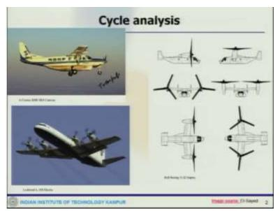
The example where top left you see, that is an example of Cessna aircraft, where this is again a turboprop engine, which is sitting there and then this one is also Lockheed. This is also turboprop based engine and also you can see these are some of these other turboprop kind of applications, which are there. So now the turboprop engines could be single, double, or triple spool. The single spool engine, the only one turbine drives one compressor and propeller.
