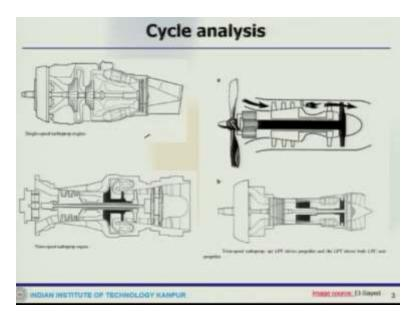
Like that would be like this is a single spool one, while it will have one single propeller or these things, then the other could be the low-pressure turbine drives either the single compressor or these and then you can have; this is a twin spool configuration. Here you can see the twin spool configuration. Here the LPT turbine drives the propeller. So here the LPT driver and drives both the LPC and propeller. This is another example.
