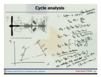
So now we can move to a two spool configuration like this where again we can look at the TS diagram quickly. This is a go to 2, 3, 4, 5, 6, 7. So this is a. So this is this is a two spool turboprop engine and again the different components can be examined here, again the gas generator where the energy balance between compressor class high-pressure turbine
