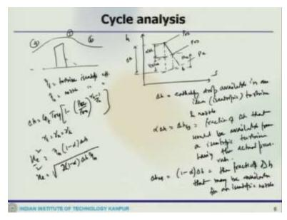
So we can look at a simple diagram to explain this like we have the turbine here. So this is 4, this is 5 and this is 6. So if we draw an diagram of enthalpy entropy diagram, so this is  $P_{04}$  where it was there coming to  $P_{05}$  and then coming down to  $P_a$ . So this is 6. So this portion is  $\Delta h$ , then this portion is  $\alpha \Delta h$ , then obviously this portion would be  $(1 - \alpha)\Delta h$  and this is called the  $\Delta h_{ns}$ .
