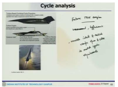
So just to conclude all these discussion with this schematic vehicle of the feature TBCC engine. So this is a Lockheed Martin SR72, which is sort of conceptualized unmanned hypersonic aircraft intended for intelligence, surveillance, reconnaissance, and this SR72 was also put to operation by 2030, because it is again what you see here, it is over-under configuration, here is the turbine engine, here is the dual mode engines and it will be based on turbine TBCC cycle.
