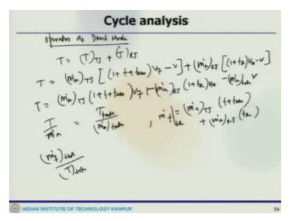
Now when it operates as dual mode, so what would happen that time? So when it operates as dual mode, then you get thrust would be of turbojet plus thrust would be combination of ramjet, then the total thrust would be
