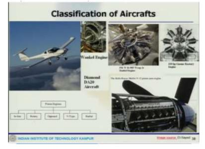
So, these are also we are going to talk, now again this was the old engine which was Wankel engine, now the piston engine has different types, so this could be inline, rotary and V type, radial type, so these are known as reciprocating engine, so this was initially or first used this piston engines. So, inline engine has cylinders I mean they are lined up in a row, it typically has an even number of cylinders.
