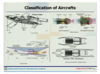
But then you have this other type of things where there is also pulse detonation engine and the this is another pulse jet engine, so this is the scramjet, here where the flow comes here with supersonic and then pass through this inlet section which would be lot of shock interaction, shock boundary layer interaction takes place and then finally it allows through combustion chamber and then finally it produces the thrust.
