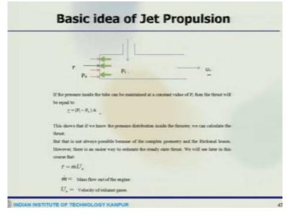
So, now if the tube is maintained at a certain pressure Pi, then the thrust would be calculated like that, so if we avoid any of these losses like frictional, so one can easily estimate that thrust which is simple way like what is the exit velocity and the mass flow rate it handles, so it is  $\dot{m}U_e$ .
