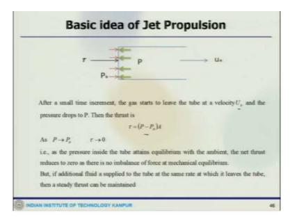
And now, when a small increment the gas starts to leave the tube, so there will be exit velocity and then the pressure drops, so you get this thrust and this pressure would move to the same pressure, if the thrust moves to 0, okay so this pressure inside the tube attains an equilibrium with ambient and the net thrust reduces to 0, okay.
