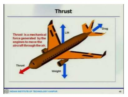
Now, the simple principle which is just to calculate the force balance and all this if you put it together in an aircraft this is what you have lift acted, weight update, drag and thrust.
