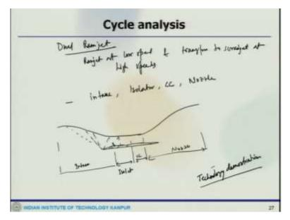
So, which is called dual ramjet so this is dual ramjet is also a dual mode ramjet. So, where the ramjet at low speed and transform to scramjet at high speeds okay. So that is how it is called dual mode. So now I mean basically this is another advancement where one can also look at these things and can do the thermo dynamical analysis that so this will also have a similar component like intake or inlet.
