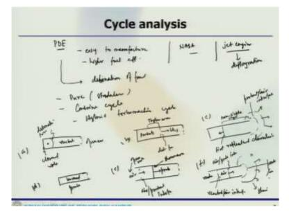
Now the one which we go of looking at the pulse detonation engine and we have since the different approach of the pulse detonation engine. So, this makes a new approach towards non continuous combustion they are also very easy to manufacture that is obvious and also having higher fuel efficiency compared to turbofan engines or something like that. Now so actually to date no practical PDE engine has been put into the production.
