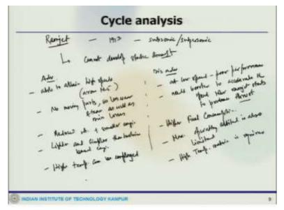
Now we will move to Ramjet so that is the so it is a another type of engine to just first proposed in 1913 by 13 so it may be either subsonic or it could be supersonic but one of the biggest problem is that with the Ramjet the thing is that the in the Ramjet it depends on the compression of the incoming air through geometric modifications. So, it cannot develop static thrust that is one of the issues with this the vehicle must first therefore cannot from the standing it cannot start.
