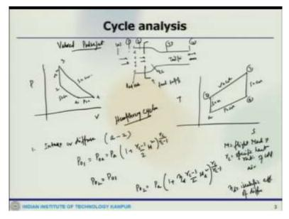
And now, if you look at that now, first we will start with the valved pulse jet and we put the simple construction of that, let us say this is how the geometry will look like, it is a simple construction where these are the; so let us say a, station number 1, this is 2, station number 3 and 4, so this is tail pipe, this is fuel supply, this is combustion chamber, so these are valve and the PV diagram would be like this is a, it goes here, then goes there, then goes there.
