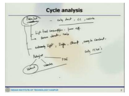
So, we will start with the engine is pulse jet, okay and then after that from pulse jet, we will move to ramjet and from ramjet, we will go to scramjet, so these are the different kind of engines where the RAM based cycles are there, so they do not have the major rotating components, so it has some sort of an entry duct and combustion chamber and nozzle, so it is that way geometrically, one can think about it they are quite simple.
