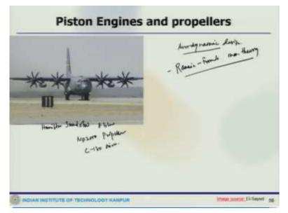
And 8 bladed propeller is here, this is Hamilton Sundstrand 8 blades NP 2000 propeller, this is used in C-130 aircraft, so there are different thing which are there like its blade, its rotation, counter rotation, now also one important factor is that aerodynamic design of the propeller because these are important how to reduce drag and so there are the way it is done is a simple Rankine-Froude momentum theory.
