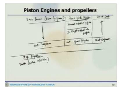
So, this is used when the typically, the hand breaks and such things fails okay, so what we can look at is that some fixed pitch versus variable pitch propeller, we can have like basic function like poor performance that could be one, then we could have fixed pitch propeller, lowest cost, okay. So and this side is the best performance, constant speed propeller and most expensive one.
