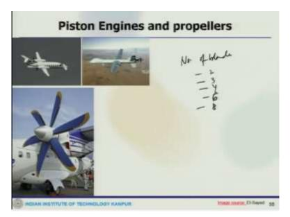
So, these are also pusher and puller, so this is number of blades where it could be; the number of blades could be 2 or 3, so let us say number of blades that could be 2, 3, 4, 5, 4, 6, 8 so multiple greater than 4 as example 8 bladed propeller which is shown here, so and this one is 6 bladed propeller which you see here.
