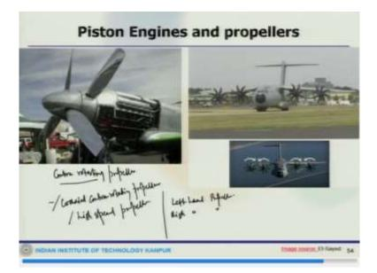
Let us see this is a double contra rotating propeller, this is a contra rotating propeller, so this is Rolls-Royce griffon powered P 55 propeller. Now, this contra rotating propeller are also called, they are also called coaxial contra rotating propeller or high speed propeller, so this apply the maximum power of an engine to drive 2 propeller in contra rotation, this rotation about the same axis in opposite direction.
