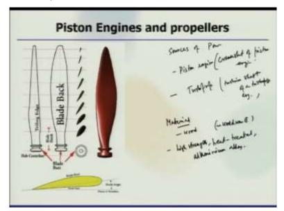
And if you want to this is a fixed, the cross section looks like this, so this is an interesting cross section, so that shows the hub centreline, trailling edge, the blade, how the airfoil shape looks like, so there are typically thick and if you see there to provide strength, so it is cylindrical
