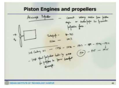
So, what aircraft propeller does or what it does is that it is actually convert rotary motion from piston engine or turboprops to provide propulsive force okay, so it may possible that so typical impeller kind of things one can think about the propeller kind of things that here it could be connected like that. So, this is a typical diagram of a propeller but this is the inlet velocity of V0.
