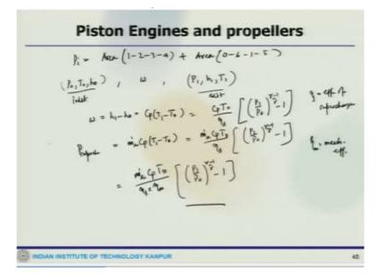
We will get  $P_i$  is that area under the curve 1, 2, 3, 4 plus area under the curve 0, 6, 1, 5, so the power required for driving the supercharger can be calculated considering the flow to be adiabatic steady. Now, the air when it enters the compressor at a pressure temperature like  $P_0$ ,  $T_0$ ,  $h_0$  and the works supplied to the supercharger is W and the when it leaves the supercharger that temperature pressure is  $P_1$ ,  $h_1$ ,  $T_1$ .
