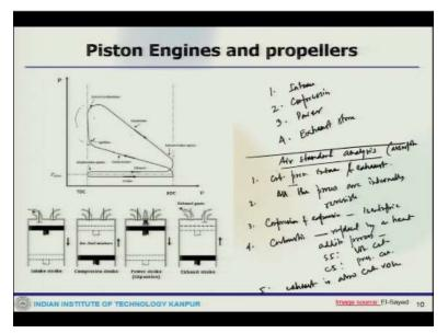
And then you can see how this happens and this is the pressure verses velocity plot. You having intake stroke where actually the valve is open; intake valve is open and the piston actually moves downward to get the fresh air inside the cylinder. For spark ignition engine this charge is combustible mixture of fuel and air and compression engine ignition engine it would be the air only.
