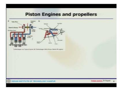
Now another type could be this turbocharger or supercharge kind of this is a Rolls Royce engines where you can see, you have a compressor then turbine wheel and how this cylinders arrangement is done and when they are; so this is a typical layout and this is a; so these are also another category of engines or this kind of intermittent combustion engines which are available for this things.
