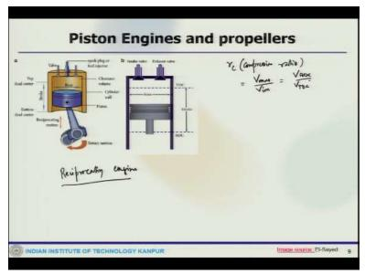
Now when you go to the Aerothermodynamics of the; let us say we start with the; so this is a typical nomenclature of any reciprocating engine. So what you have, you have cylinder which is connected with the crankshaft here and the crankshaft which rotate so this cylinder with the piston head, a cylinder with this piston actually moves up and down which creates this reciprocating motion and then there are spark plug, there are valve which is use for the intake and exhaust.
