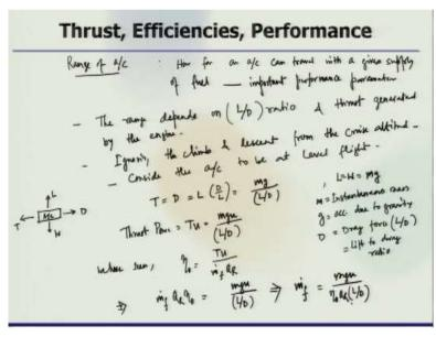
So, what we will discuss is the range of aircraft. So, that is we are going to look at it. So the range when we talk about range it means it says how far an aircraft can travel with a given supply of fuel. Given supply of fuel so this is also an important performance parameter and range actually the range depends on L / D ratio which lift to drag ratio and thrust generated by the engine.
