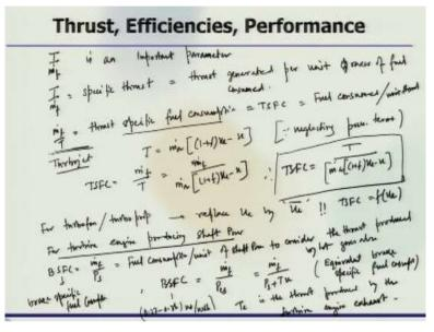
So which tells that  $\frac{T}{\dot{m}_f}$  is an important parameter. So  $\frac{T}{\dot{m}_f}$  is an important parameter and this is the specific thrust that means the thrust generated per unit mass of fuel consumed. Now the other the reverse of it which is  $\frac{\dot{m}_f}{T}$  this is called the thrust specific fuel consumption that is TSFC that means fuel consumed per unit thrust. So just to produce one unit of thrust how much fuel is consumed that is called the TSFC.
