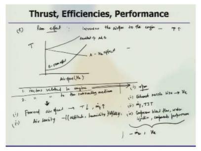
Then we can have let us say another one in that continuation is the Ram effect. So, this is something that movement of the aircraft which is relative to the outside air which causes some air to be ramped into the engine inlet duct. So what it does the ram effect actually increases the airflow to the engine which in turn increases the gross thrust. However, it is not easy that ram effects combine two factors.
