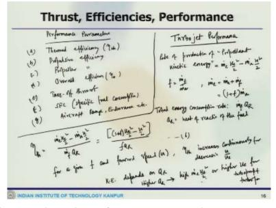
Now we would sum up the engine performance parameter that we can categorize or look at some efficiency like thermal efficiency which is designated at eta h. Propulsive efficiency, propeller efficiency, overall efficiency then take-off thrust then SFC which is specific fuel consumption then obviously range and other factor. So we can put it aircraft range, endurance etcetera.
