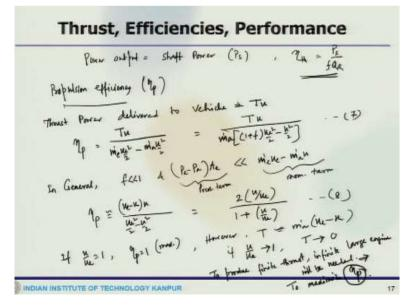
So the power output is nothing, but the shaft power which is let us say Ps then one can write thermal efficiency as Ps / fQR. So that means what is the power output and what is the energy
