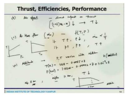
And then we have talked about air speed and then air mass flow rate how that is connected with the pressure and temperature then the altitude obviously altitude variation that will have serious impact.
