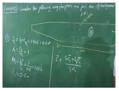
Consider the following wing planform right and find the aerodynamic center. Yeah, find the aerodynamic center. That is good enough, all right? So this is what the planform is. We have a rectangular portion of this wing, right in the center. Let us say this is my f RL, fuselage reference line that we discussed earlier. So let us consider a rectangular wing. So have a rectangular wing portion in between.
