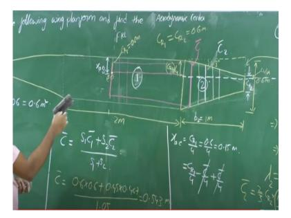
So if you substitute that what we have is C bar is equals to 0.6 times 0.6 plus 0.45 multiplied by 0.467, right upon 1.05. So what you have is C bar is equals to 0.543, 0.543 meters approximately. So 54 centimeters is the mean aerodynamic chord. So here we have 60 centimeter. So this mean aerodynamic chord will be somewhere here right, which is 54 centimeters, right.
