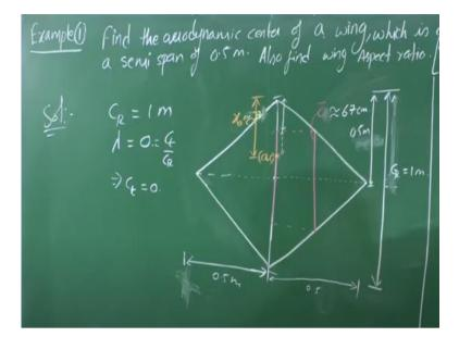
The wing is a flat plate. So from the question we can tentatively get some rough idea about the wing planform here. So we have root chord which is about 1 meter and the taper axis is so that is 0.5 meters. Am I correct or not? Say if this is my root chord, which is 1 meter and the midpoint should be 0.5, right. So and I was given the information about semi span, right.
