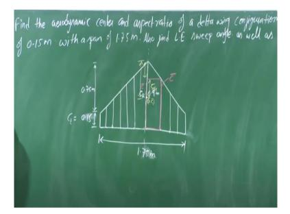
So find the aerodynamic center and aspect ratio of a delta wing configuration with a root chord of 0.9 meters and tip chord of 0.15 meters with a span of 1.75 meters. So this is what we have. So we were asked to find the mean aerodynamic center, location of aerodynamic center, mean aerodynamic chord. Yeah of course, to find out aerodynamic center we need mean aerodynamic chord and the aspect ratio of a delta wing right.
