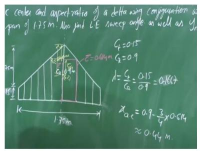
So we know C t is equals to 0.15.We have C R is 0.9. So lambda is straightforward C t upon C R, which is 0.15 over 0.9, which is approximately 0.1667, yeah. That is taper ratio. So if I substitute that is 1.1667 plus 0.1667 square upon 1.1667, right. So if we solve this so this is equals to 0.614 meters, okay. This is the mean aerodynamic chord.
